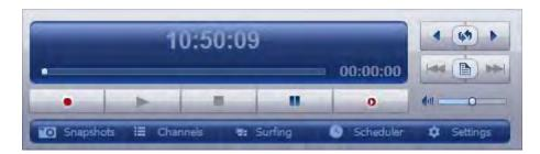
**Display** – shows current time or time elapsed since the file recording or playback started and also the real-time delay during the time shifting process. It also shows the process state and the name of the channel you watch or record.
